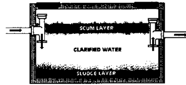
Treated Free-Flowing Septic Tank
